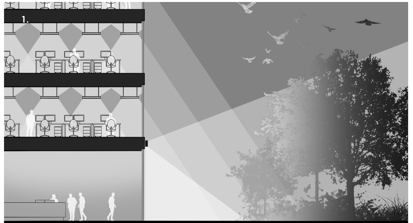
1. Glazed façades without treatment and external lighting with insufficient optical control can cause light trespass intrusion into green areas spaces and potentially create bird strike.
